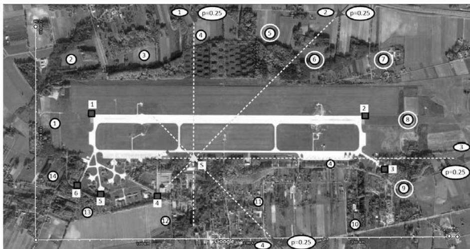
Fig. 3. Illustration of the optimum AAMA set displacement points around the protected area for the airfield under different air raid variants. The air raid variants vary in the probability of air target emergence for specific air raid direction.
