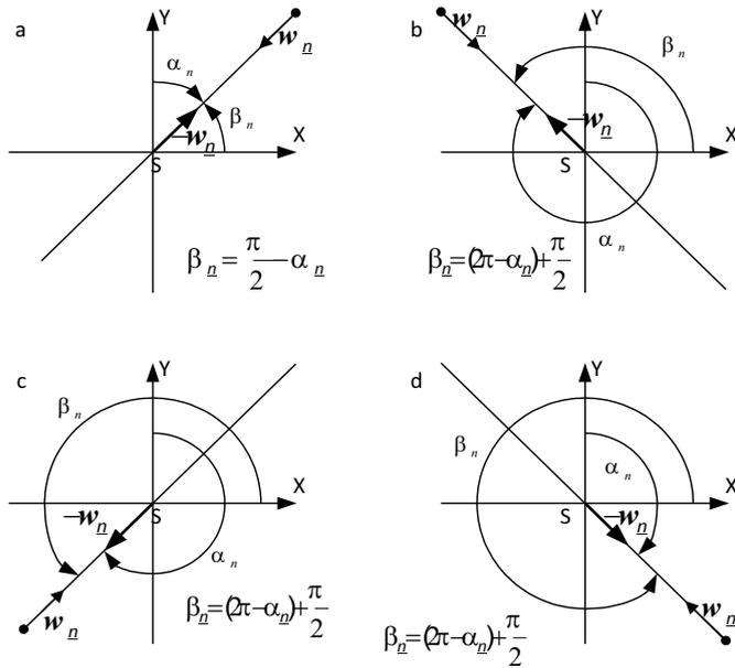
Fig. 1. The interrelations of air raid direction, air raid direction unit vector  $w_n$ , air raid direction azimuth angle  $\alpha_n$  and air raid angle  $\beta_n$ .
