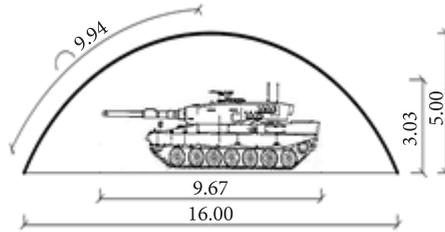
Fig. 5.1. Cross-sectional diagram of the medium-sized dome
