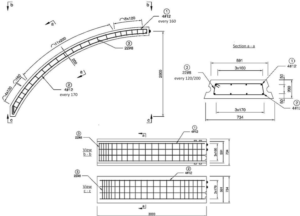
Fig. 5.3. Form Type 1 module structural reinforcement [3]
