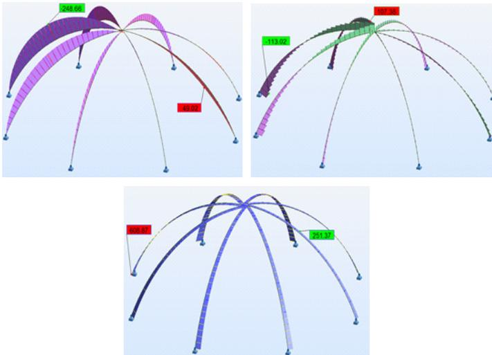
Fig. 5.2. Charts of internal forces: (a) bending moments [kNm]; (b) transverse forces [kN]; (c) axial forces [kN]; [3]
